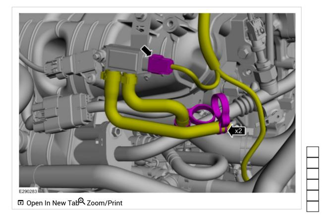
2. Remove the fastener and differential pressure feedback EGR sensor. *Torque* : 97 lb.in (11 Nm)
