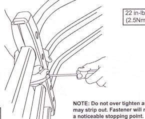
NOTE: Do not over tighten as this may strip out. Fastener will reach
