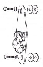
Install Pivot Brackets to upper two threaded holes on D-Pillar. Each bolt location will take two plastic spacers (4 total per bracket, as shown) under the bracket to properly space
