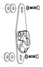
Passenger side, Bracket and hardware orientation
