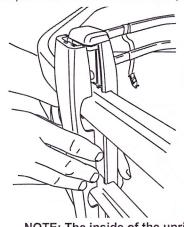
Upright is not positioned in center of tube joint.
