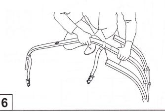
Insert the top long tube into the top tube of the 3-tube assembly.
