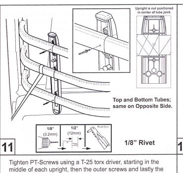
Attach plastic upright around the tube juncture, placing rubber bumpers into the two ends of the upright.
