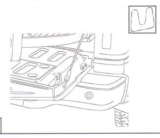
Adjust Strap Buckles to lock into the tailgate when Bed Extender is deployed.
