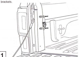
Tighten fasteners. Make sure pivot opening in bracket opens towards the rear of the vehicle.
