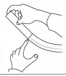
Slide the center tube into the center tube of the 3-tube assembly. Straps will be pre-assembled to center tube. Insert tube until edge of unpainted section meets mating tube.
