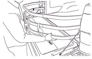
Note: Make sure straps are allready installed on center tube before completing assembly.
