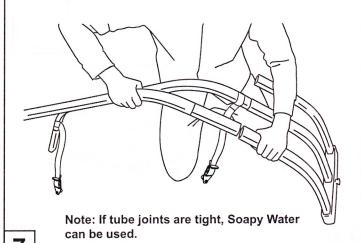
Insert the bottom long tube into the bottom tube of the 3-tube assembly.
